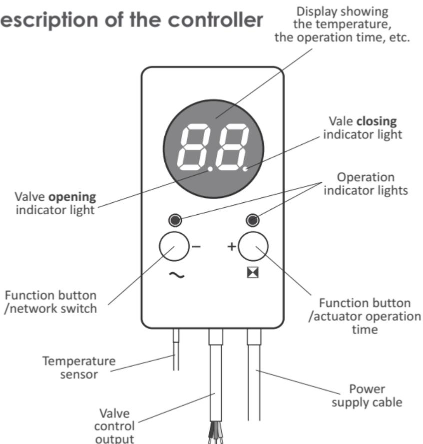
*The valve **opening and closing** indicator lights indicate the status of operation of the actuator. Blinking indicator lights indicate operation of the valve to the left or to the right.*
