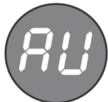
When the “AU” value is set, the controller will resume operation in the automatic mode (an actuator with limit switches).
