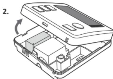
The lead terminals are on the controller's back wall, under the plastic cover.
