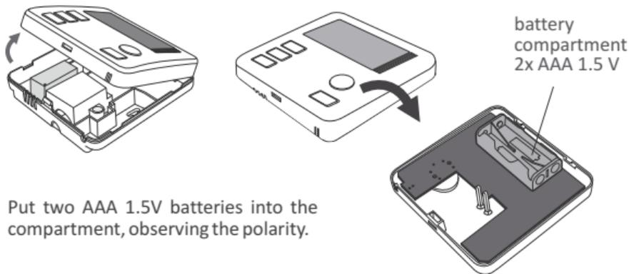
Put two AAA 1.5V batteries into the compartment, observing the polarity.
