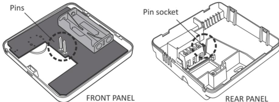
When replacing the front cover make sure that the pins are inserted into the pin socket.
