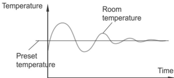
With these values determined, the controller switches the heating device on and off in cycles that enable maintaining temperature as close to the setpoint as possible.
