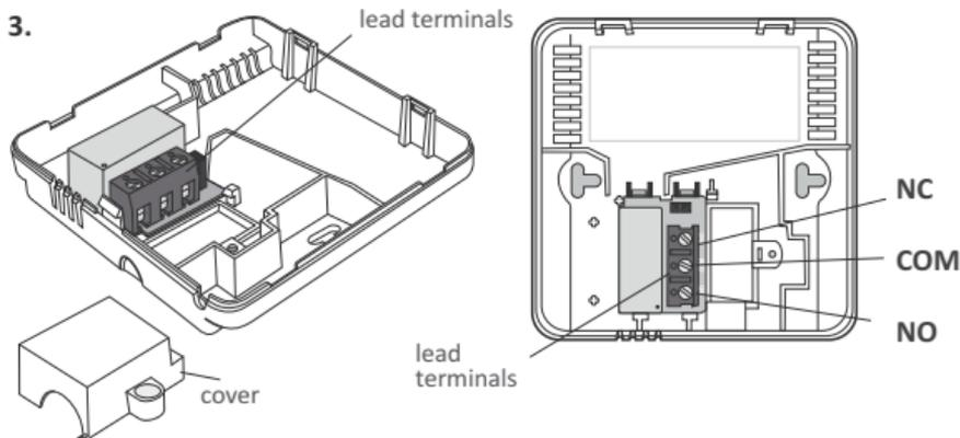
It is a typical single-pole two-state relay. In most cases, the NC terminal is not used.
