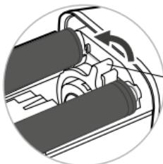
**f)** Turn the safety ring into the "secured" position.
