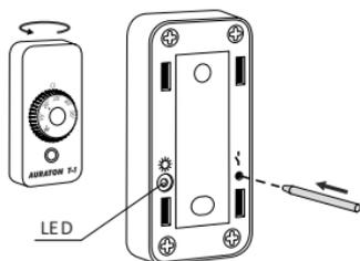
2. Press the pairing button (▽) placed on the rear side of housing and hold it for about 2 seconds. When LED diode (⚡) will starts flashing red stop pressing the button.
