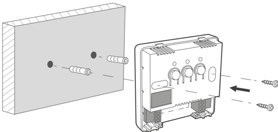
**NOTE:** If the wall is wooden, there is no need to use wall plugs. In such a case, drill two holes 2.7 mm in diameter instead of 5 mm, and screw the screws directly into the wood.
